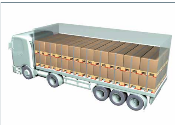
Correct load securing: anti-slip mats are coloured red.
