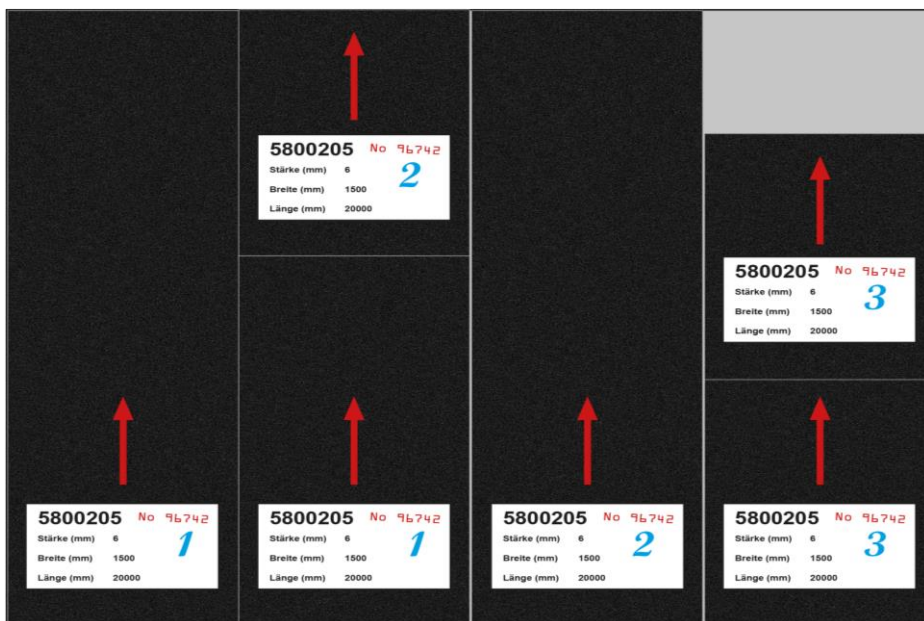
Rolling out the consecutive rolls in the same direction
