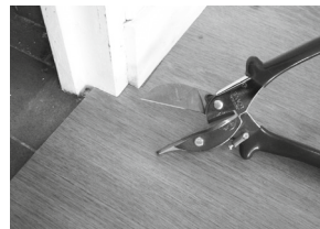
Mitre shears Reference : Romus : 93415 / Janser : 237 530 000 For cutting around door frame bases and areas which are difficult to access.
